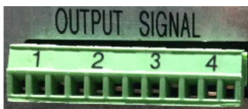
Figure 3-17, Output signal connector
